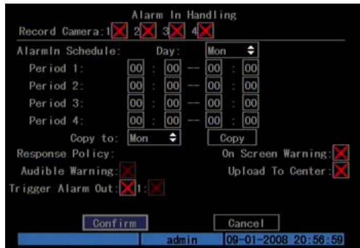
Fig. 5.24 Alarm in handling setup
